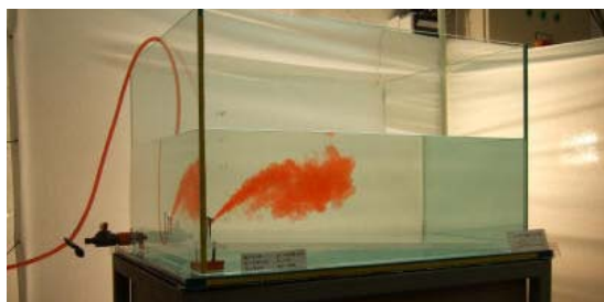
Fig. 3: Left: Laboratory setup to visualize a dense brine discharge resulting from a RO plant (Niepelt, 2008); Right: Modeled dense discharge with CORMIX.
