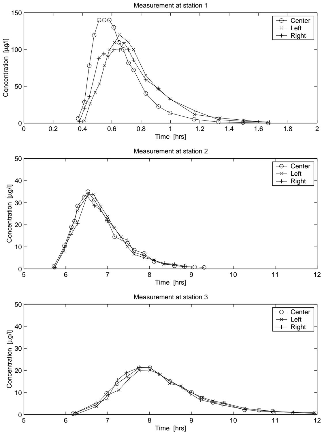
**Fig. 3.7.** Measured dye concentrations at two stations in Cowaselon Creek for a point injection. Measurements at each station are presented for the stream centerline and for locations near the right and left banks.
