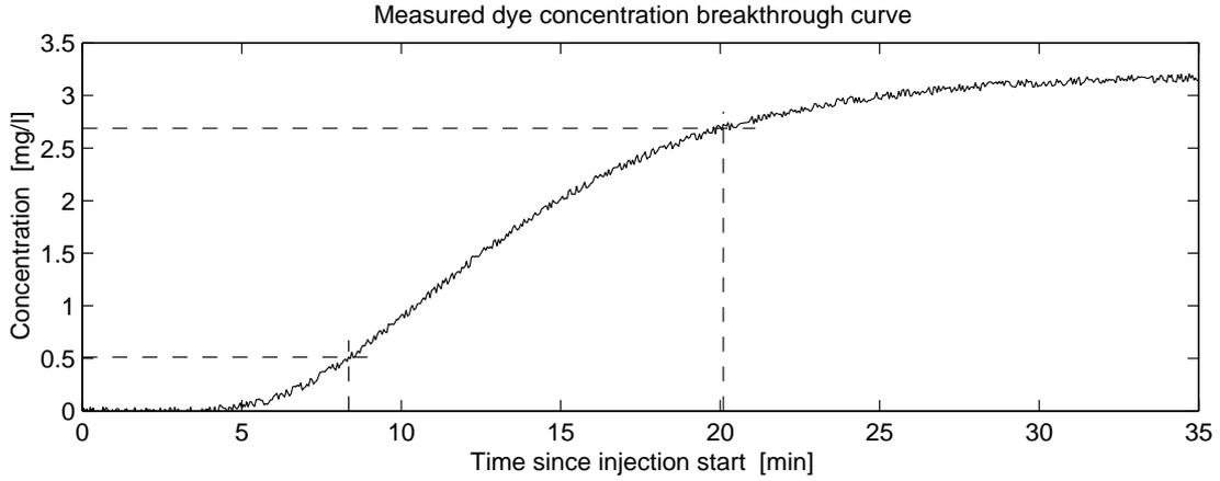
**Fig. 3.6.** Measured dye concentration for example dye study. Dye fluctuations are due to instrument uncertainty, not due to turbulent fluctuations.
