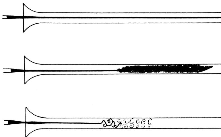
**Fig. 3.1.** Sketches from Reynolds (1883) showing laminar flow (top), turbulent flow (middle), and turbulent flow illuminated with an electric spark (bottom). Taken from Acheson (1990).
