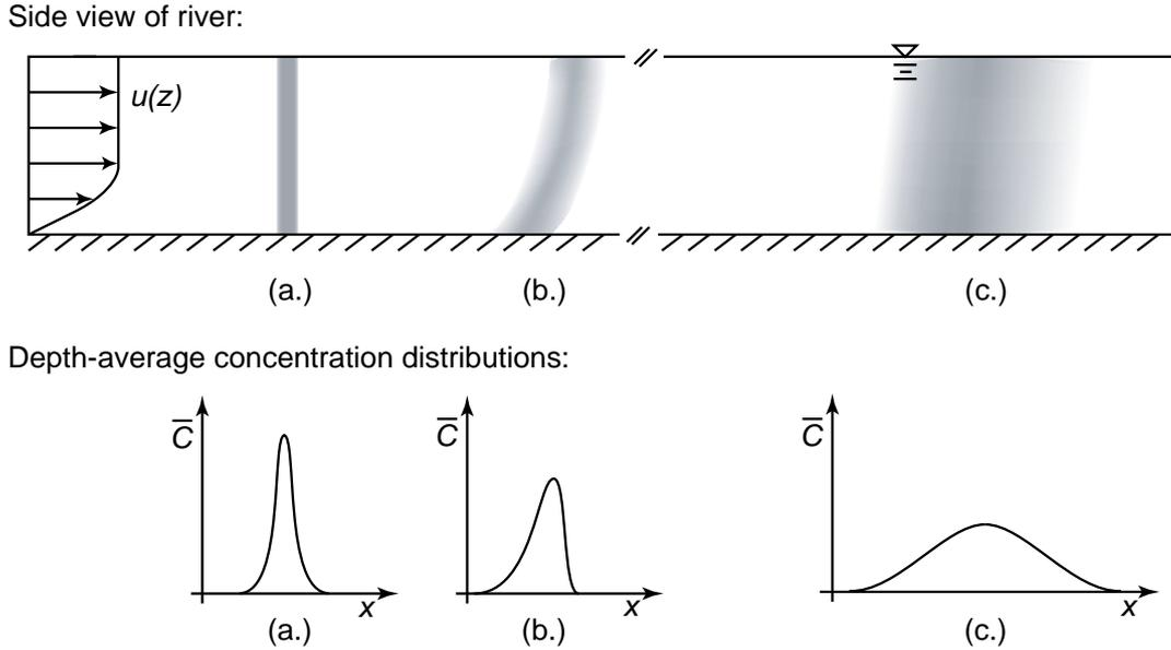
**Fig. 3.3.** Schematic showing the process of longitudinal dispersion. Tracer is injected uniformly at (a) and stretched by the shear profile at (b). At (c) vertical diffusion has homogenized the vertical gradients and a depth-averaged Gaussian distribution is expected in the concentration profiles.
